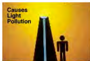
This diagram shows a lighting fixture that throws light upwards and sideways.
